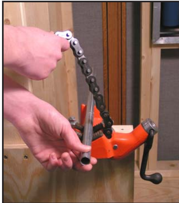
Placing the Pipe in the Chain Vise
